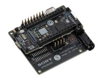
Sony's SPRESENSE microcontroller with LTE Connectivity from Soracom
